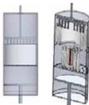
Picture 1: Front View of the Detector. There is a Solid Moderator Chamber at the Top, a Measuring Chamber at the Middle and a Liquid Moderator Storage Chamber at the Bottom.
